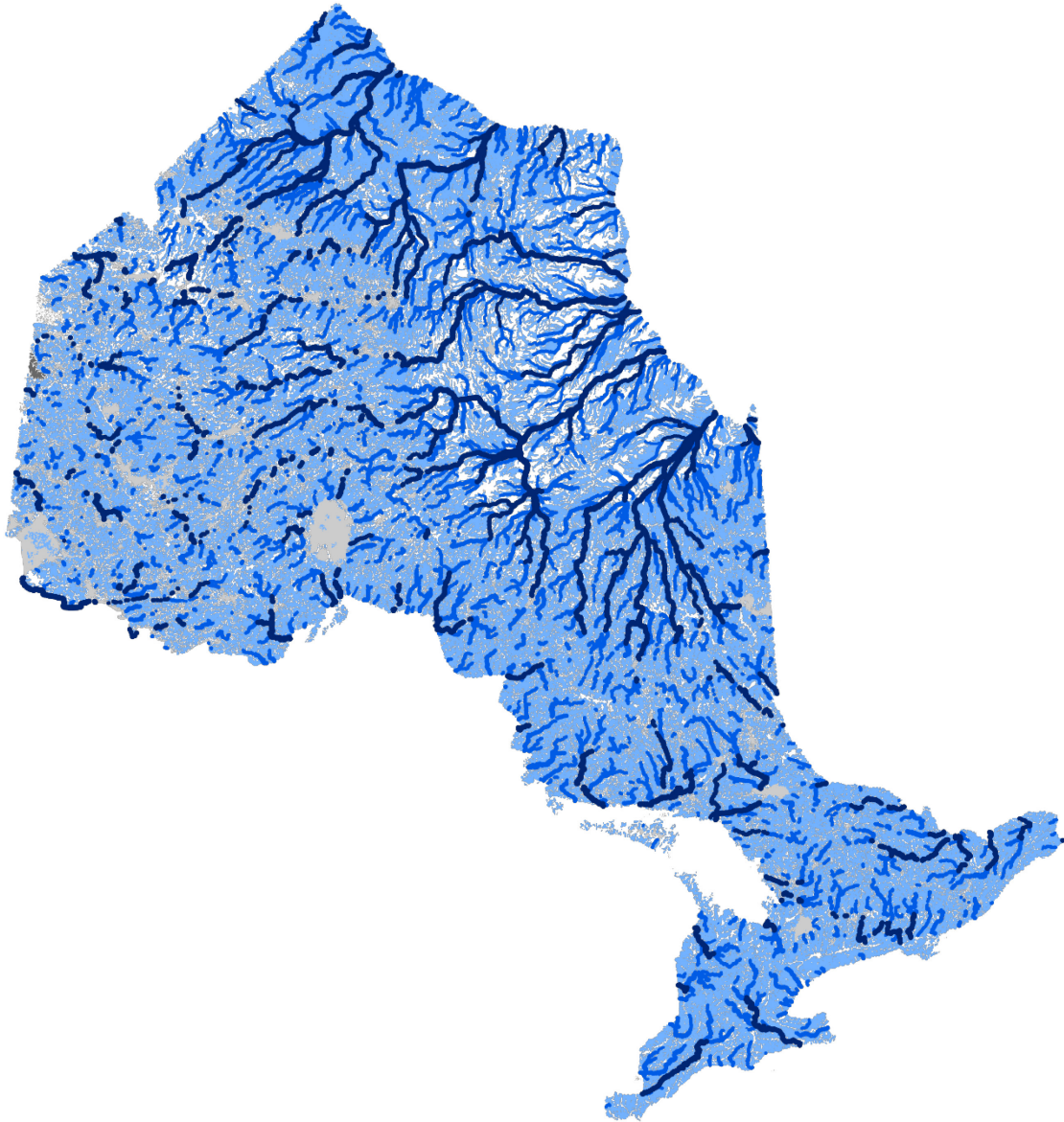
Figure 13. Based on drainage area, three categories of stream size in Ontario are wadable streams (<200 km 2 , light blue), non-wadeable streams (>2,000 km 2 , dark blue), and intermediate streams (≥200 to <2,000 km 2 , medium blue).
